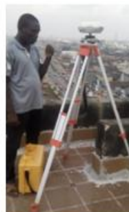
Fig. 6: Rover receiver at Monitoring point M
